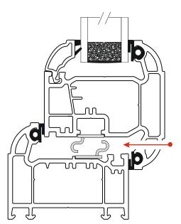
**STAY GUARD ELITE SG035** on outer frame and sash for types of stay to include Egress/Easy Clean
