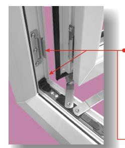
Fit Stay Guard Elite approx 75mm centres from the internal corner as show here. Secure using 4.8 X 25 carbon steel zinc coated
